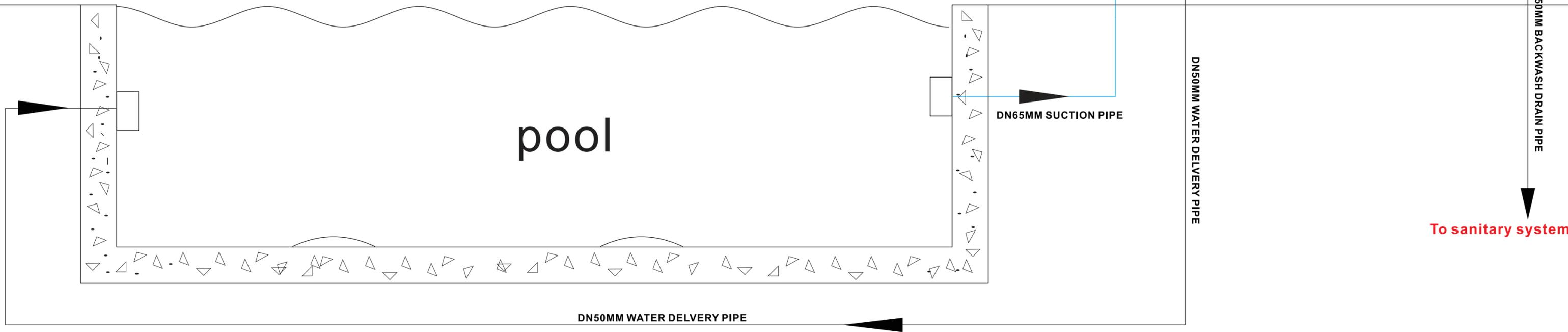
Schematic diagram of MOB filtering system
